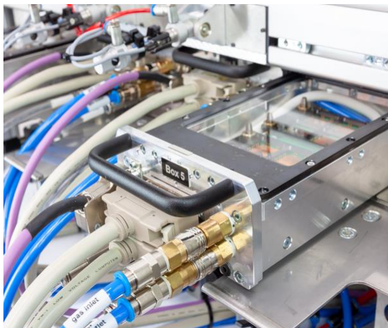
Contacted Probe-box HySprint infrastructure (© HZB)
