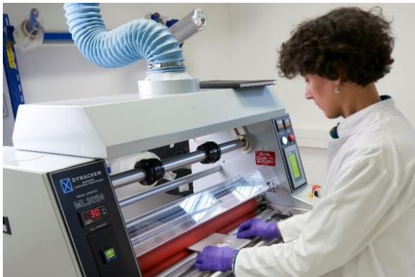
Lab roll to roll laminator (encapsulation) @CEA-LITEN
