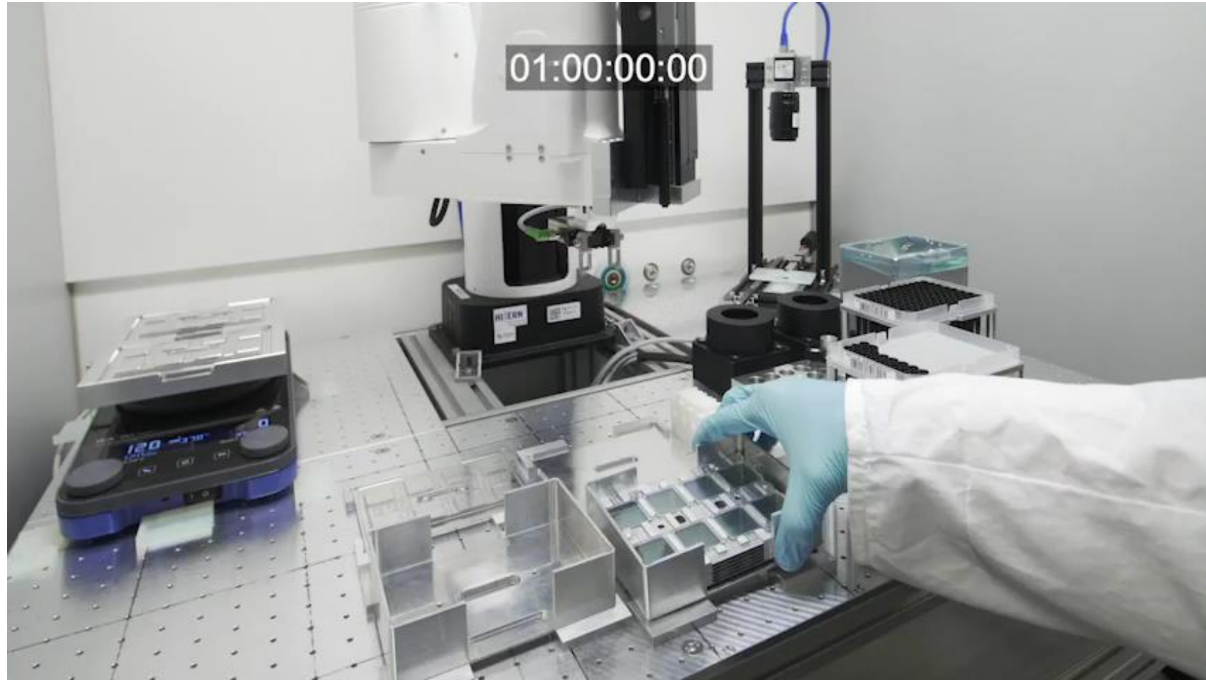
Scara-Robot (1), Gripper (2), pipetting channel (3)
