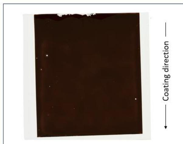
**Figure 13.** Optical scan of the perovskite layer slot die coated on a 6-inch PET/ITO substrate. The perovskite layer is coated onto the SnO<sub>2</sub> layer.
